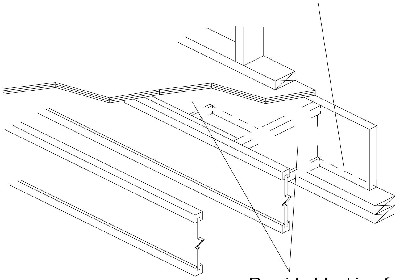
Provide blocking for lateral support as required. Use LP I-Joist, LP LVL, LP LSL, or LP Rim Board as blocking
