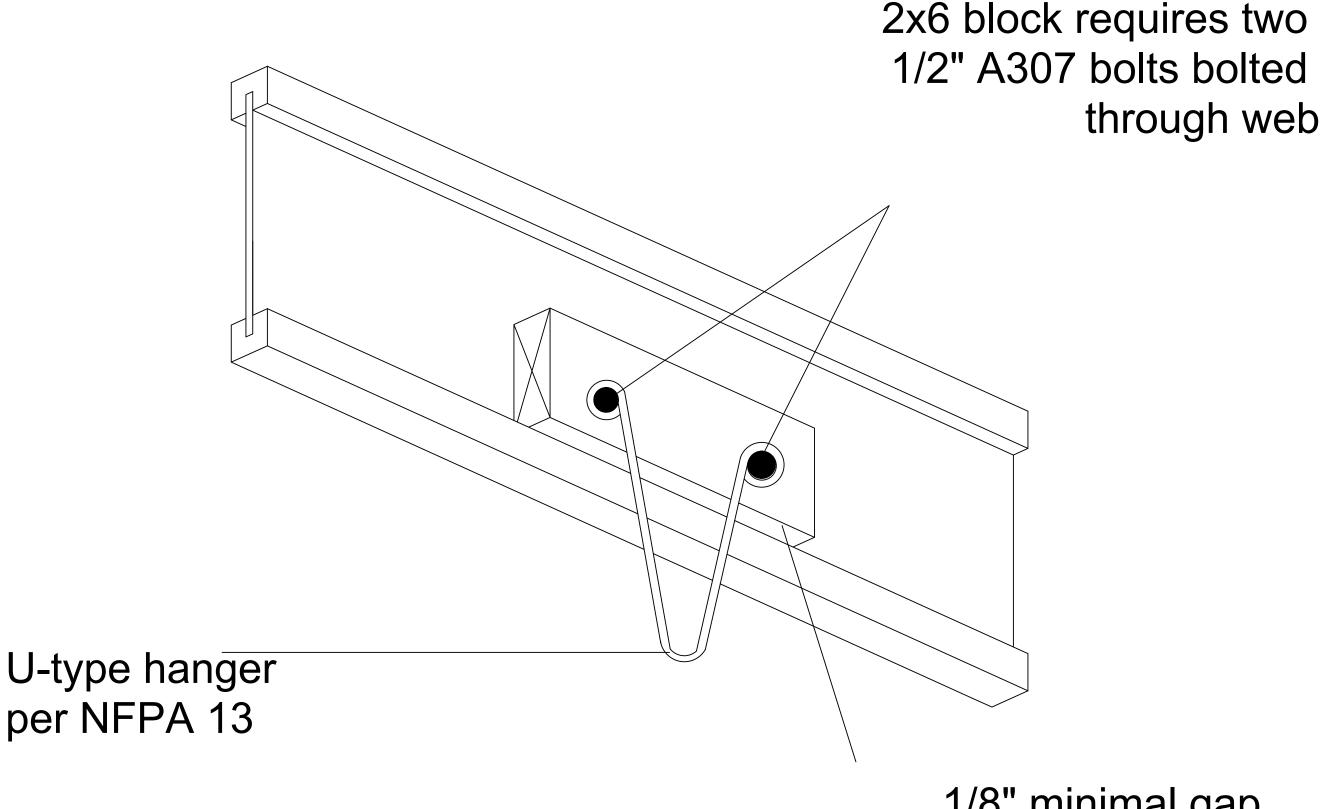
1/8" minimal gap between block and flange
